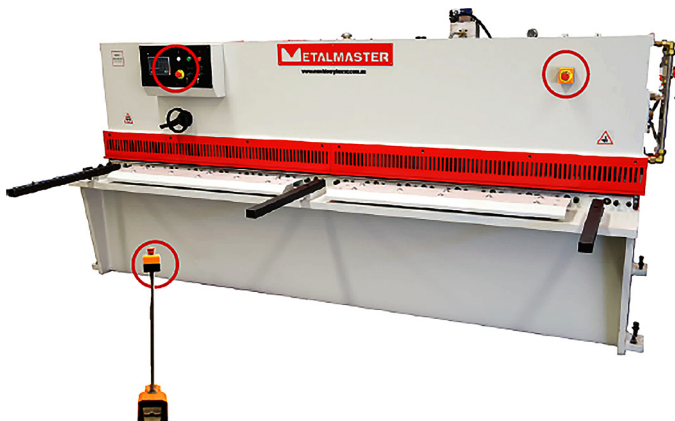
Emergency Stop Buttons
