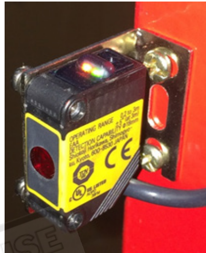
Has Power & aligned ok
